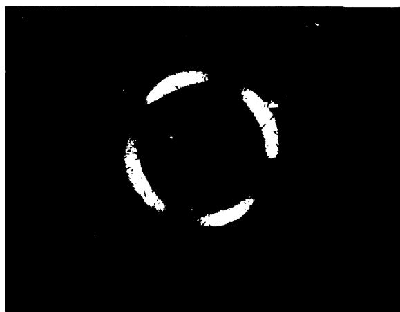
FIGURE 5 (a) Schematic representation and (b) photograph of a circular planar waveguide based on PVCi films [9].
