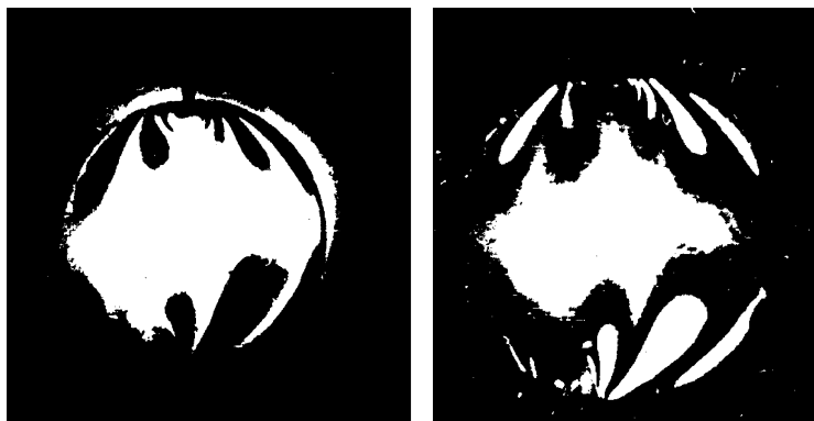
FIGURE 10 Two different positions in crossed polarizers of the exposed PVMCi film with the image of the transparent model in the deformed state. The phase image provides a visualization of internal deformations.
